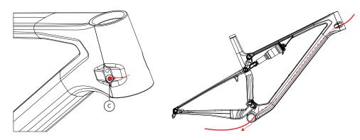
3.5 Insert the cable through the hole in the central coupling (adapter) in the saddle tube.
