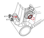
3.6 Slide the cable through the cable tube out.
